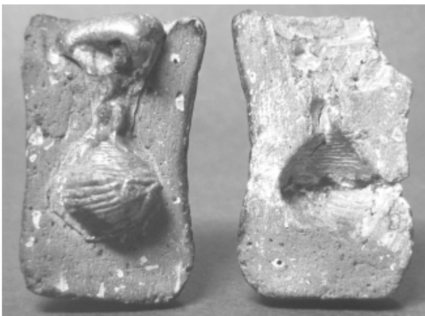
Fig. 13 Lost-wax casting mold refilled and opened. Museo del Oro, Bogotá. H. 5.7 cm.
